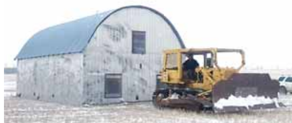
Bray used his D7 dozer to move this 25-ft. by 40-ft. barn over a mile and a half.
