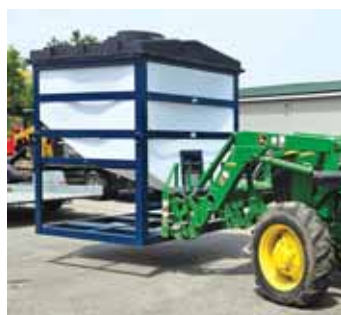
Bins are mounted on the frame for easy filling of 5-gal. pails. The different models that are now made are rated in bushels.
