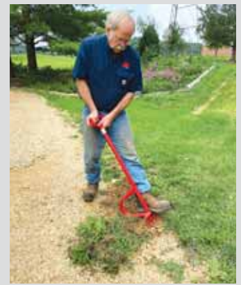
EarthLifter uses a rolling fulcrum for leverage to take the heavy work out of digging plants and roots.
