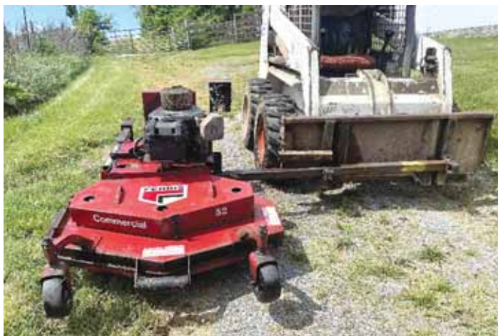
To secure the mower to the skid steer, Wampler mounted 2 1/2-in. square tubing under the main frame of the deck and to the loader bucket. He designed the mower to be pushed or pulled by the skid steer.
