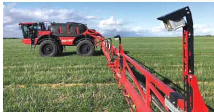
Existing sprayers can be retrofitted with the technology to apply herbicide to only the weeds rather than spraying a bare field or the entire crop.
