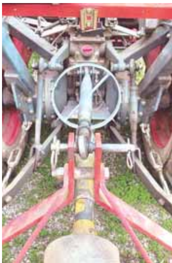
Beggs located an old steel wagon wheel about 1 1/2 in. wide and just over a foot in diameter. He had a friend attach the wheel rim onto the top link, adjusting the bracket by welding two metal rods to the bracket and the rim.
