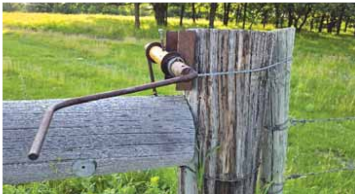
Grovom's gate closer ensures a tight gate without using a fence stretcher.
