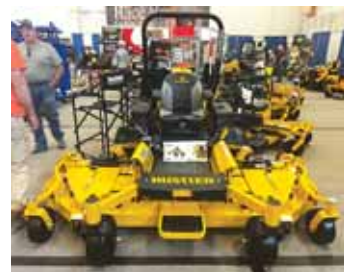
Hustler mower features a 104-in. deck and can mow at speeds up to 11 mph.
