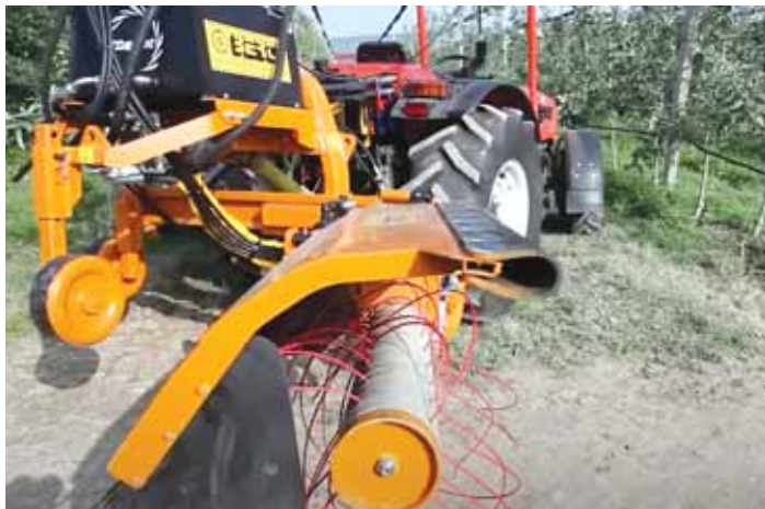
Each of the 16 sections contains a spool of cord that feeds out automatically. The spools can be quickly reloaded by hand or with an optional mechanical winder.
