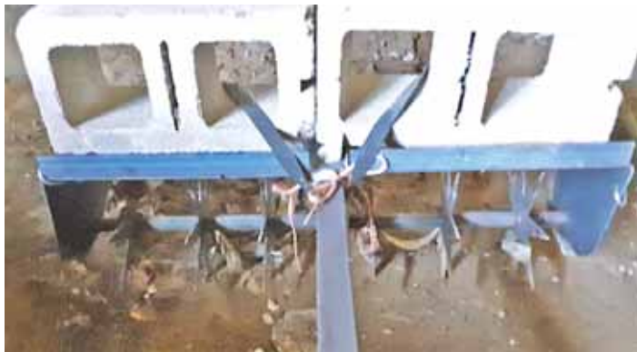
Miller used 10-gauge steel for most components, including the 8-point aerating blades, cutting them out on his CNC table.
