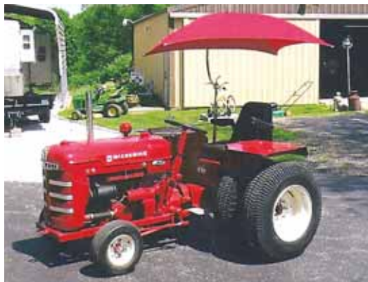
Zook built a custom tractor using an old IHC combine engine mated with a Ford truck transmission and Ford car rear end.
