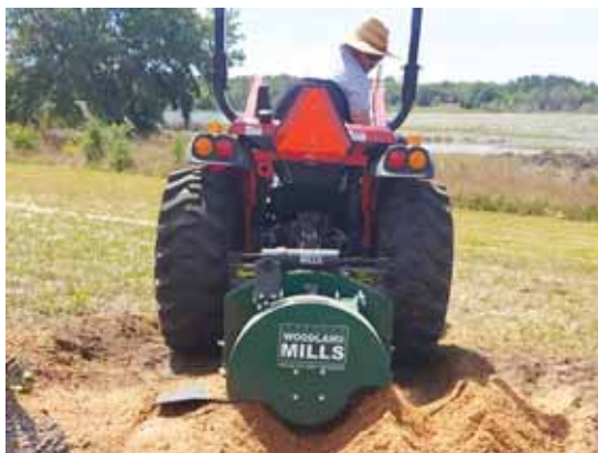
Stump grinder can dig up to 8 1/2 in. below ground.
