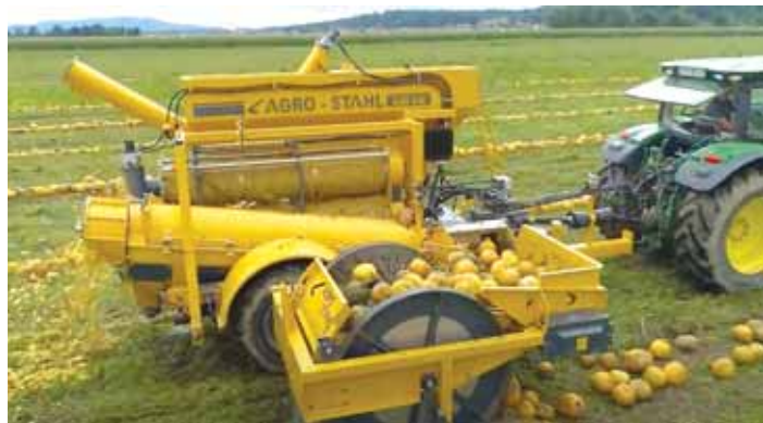
Harvester has variable speeds for operation and cleans seed during threshing.
