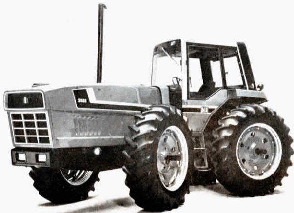
Rear half of new 4 wheel drive tractor is same as that used in the current IH 86 series tractors.
