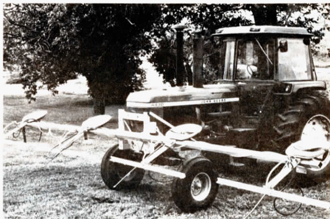
Each rider operates an 18-in. spray gun. Rig will also broadcast spray at all or any one station.
