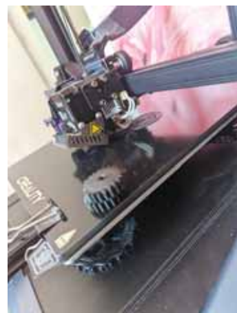
3D printer used to make replacement gear that was no longer available.
