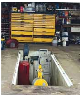
Gray lined his oil change pit with LEDs and has a platform he can slide over the pit when not in use.
