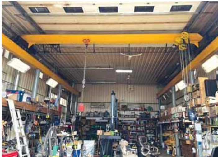
16-ft traveling crane with a rolling hoist was added to the rebuilt shop.
