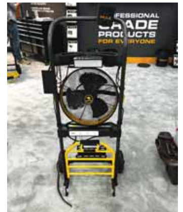
5-in-1 Mobile Workshop has an integrated 3-speed fan, LED light, power strip with a 10-ft. cord, tool caddy and 300-lb. capacity hand truck.
