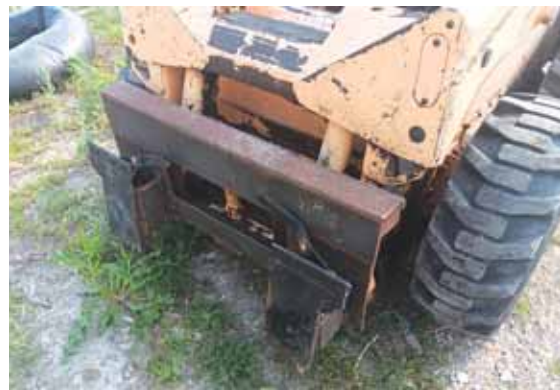
Bowen built his converter so he could use Bobcat style attachments with his Mustang skid steer.
