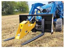
Worksaver's EPFC-1 is designed for subcompact and compact tractors up to 48 hp. with Class 1 fork attachments.
