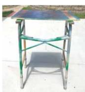
Nonhof cut off the plastic hand grips on each side of the walker to create a solid surface for bolting the boards. "I used a 1-in. by 2-in. board bolted to the walker hand grip area," he says.
