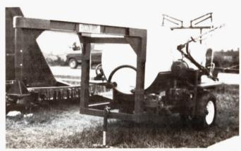
Yocum "gooseneck" sprayer has ground-driven metering pump for delivering uniform amount, regardless of field speed.
