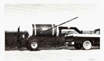
Boom height on the Otho Clark gooseneck sprayer is adjustable in height from 1 ft. to about 4 ft. off ground. Just-introduced model is equipped with a 500 gal. tank for spraying, or for applying liquid fertilizer.
