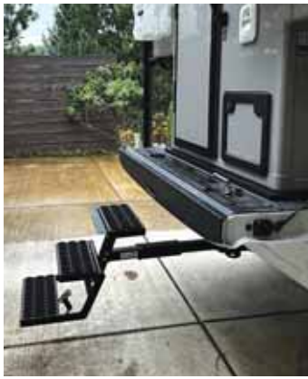
Black, foldable, textured, powder-coated step treads measure 7 by 15 in. and weigh 32 lbs.
