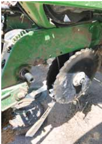
PTT’s Sabre Tooth propels the blades forward, causing less hair-pinning and minimizing sliding. The company claims their blades turn 92 to 95 percent of the time during forward motion.
