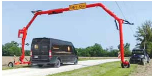
The 25-ft. upper horizontal pipe reaches across most standard 24-ft. roadways.
