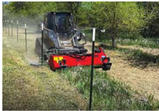
An operator moves the disk into position with a cab-mounted switch. It cuts under fence wires and pushes up against posts or trees.
