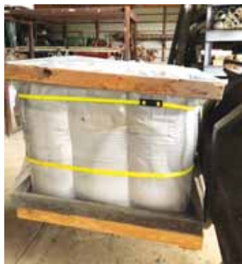
Doerr came up with the idea of putting a cap over the top of the bag where the material is the thinnest and then using strings to tie up the bag.
