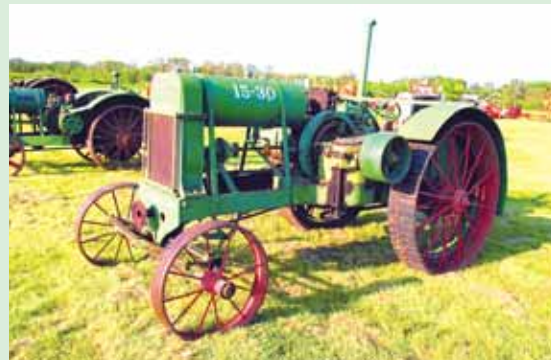
The "New Hart Parr" was a tractor equipped with a two-cylinder, slow-speed, water-cooled engine with force-feed lubrication and open gears used to drive the rear wheels.
