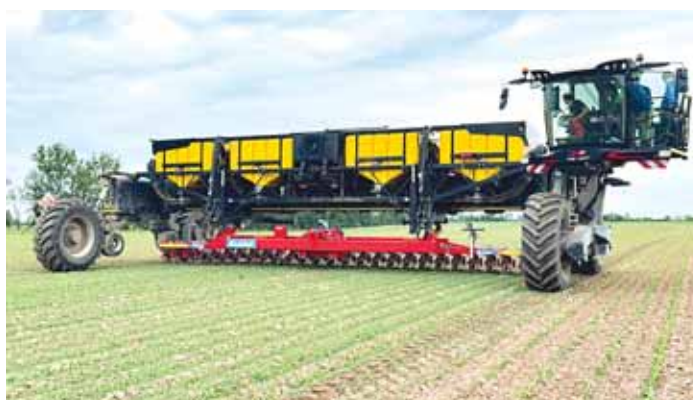
Einböck, an Austrian implement company, produced a 50-ft. wide weeder spaced for 20-in. rows to mount on the Nexat carrier system.
