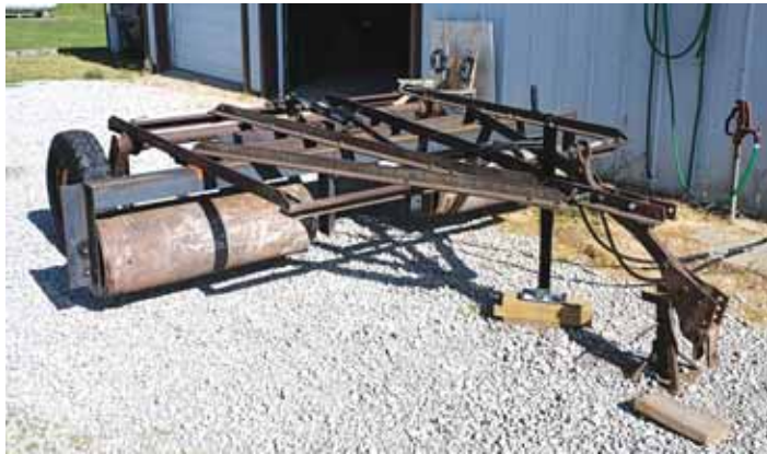
Machande used a 10-ft. disc frame and three old 100-lb. propane cylinders to make his cultipacker.
