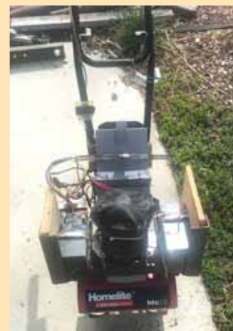
Front view showing lead-acid batteries.
