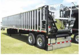
Aluminator trailer, with its hydraulic floor speed control, is designed for unloading in as little as 3 min. The floor has a 3/8-in. thick UHMW plastic liner, and the sides are lined from the bottom to the top with 3/16-in. HMW plastic.
