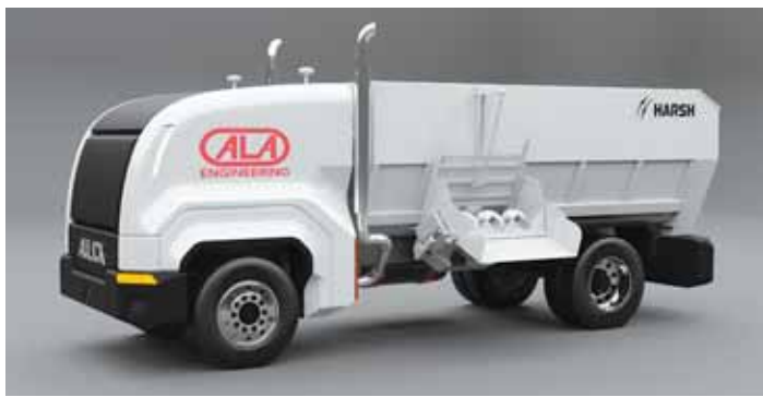
Artist's rendering of ALA Engineering's cabless, autonomous feed wagon.
