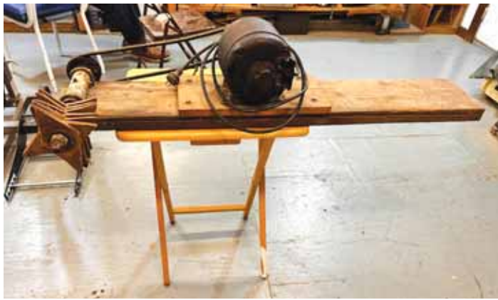
Materials for the plucker included a mandrel/head made out of a handrail filled with grease, along with two bearings pressed on each end.
