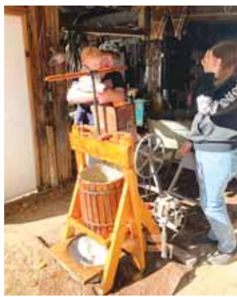
Cider press with motorized grinder, hopper extension and mesh cone-shaped screen.
