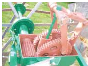
Fully restored mill with recast parts connected to the wheel.
