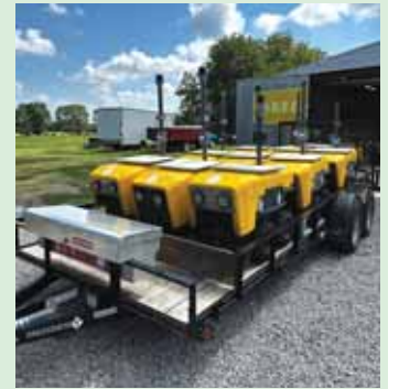
Robot's size minimizes field compaction as are designed to fit between 30-in rows.
