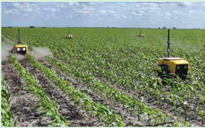
Robot fleet in action weeding a field.
