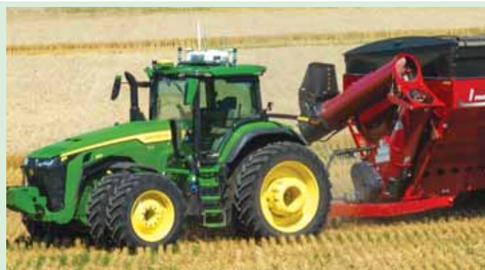
"With the OutRun kit mounted to the roof of the grain cart tractor, the combine driver can call the tractor to them to fill the grain cart on the go and then send it back to the semi's staging area," says Subramaniam.
