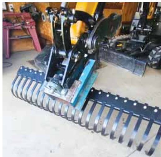
Carolla built a heavy-duty box bracket that lets him quickly attach and detach different tools to his mini-excavator.
