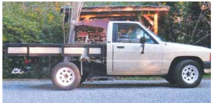
Bodman bolted the 5 by 7-ft. bed to the truck frame. He installed LED taillights and new roofing metal for the floor.
