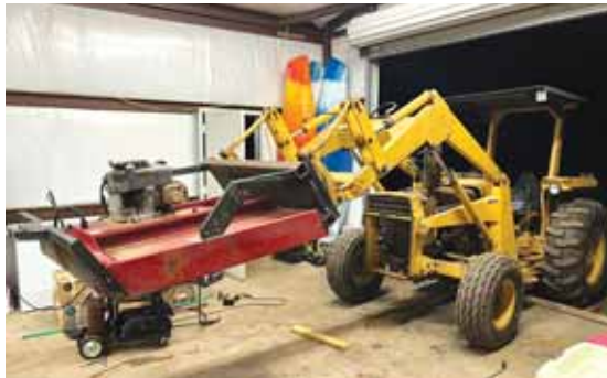
Tomamichel designed and welded mounts, adapters, supports and braces to fit his loader and connect to the quick coupler.
