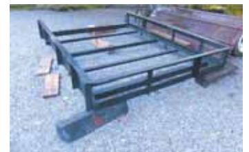
Original trailer bed was 5 by 8 ft., then cut with a grinder, welded to 5 by 7 ft., then mounted to the truck frame.
