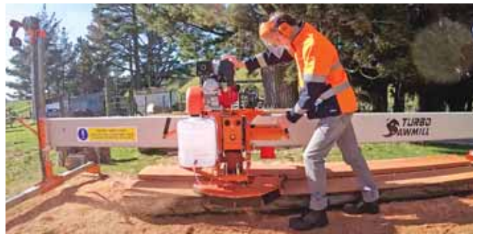
Turbosawmill offers multiple models, with standard cuts ranging from 6 by 6 in. with the M6-13M to 12 by 12 in. with the M12-28A.
