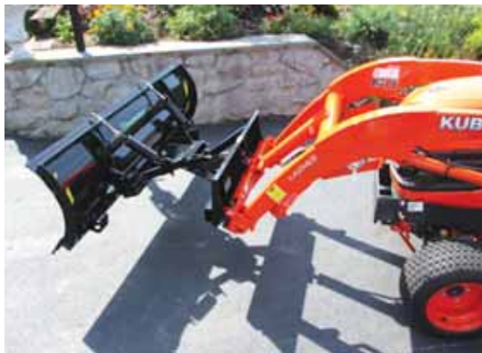
Installing the blades doesn't require any bucket alterations. "Our clamp-on plow design is unique; they clamp onto the bucket with a full underframe and two top clamps, making the bucket stiffer," explains Bentley.
