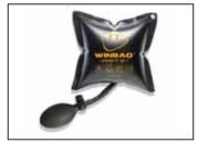
Gary F. Thomsen, Arion, Iowa: Gary nominates WINBAG as a best buy (https://winbagusa.com; ph 941-404-6064). "WINBAG is a 6-in. by 6-in. bag with an attached short tube and squeeze ball. It's made in Denmark. When the ball is squeezed, the bag expands up to about 2 in. thick. It'll lift 300 lbs. Use it in place of shims to install doors, windows, appliances, cabinets, etc.
