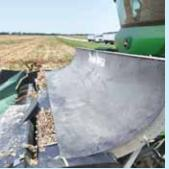
Tipper is controlled by key-fob remote and can be installed in less than an hour.
