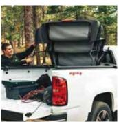
The interior and fully integrated bow system provide clear-span access. When not needed, the entire top folds forward into built-in storage at the front of the bed.
