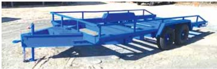
"I mounted the frame on 7,000-lb. tandem axles, also salvaged from a house trailer," says Sieting. "I cut out the original mobile home brakes and put in replaceable brakes."
