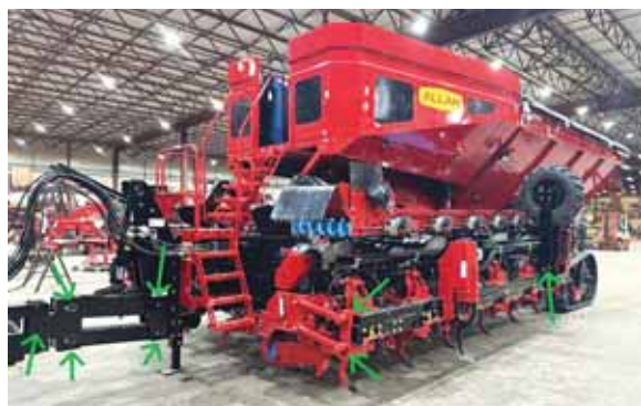
High-capacity 12-row planter can plant 10 sets per second at 7 mph.
