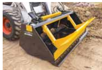
Equipping a skid steer with a Push-Off Bucket immediately increases the dump height by 3 ft., as does forward dumping.
