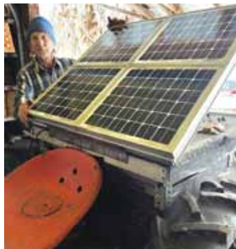
Galazyn made the electric tractor even more efficient by adding solar panels mounted over the battery box behind the operator's seat. He also made a rack to hold four 2-sq. ft. panels that he can raise to match the sun's angle.
