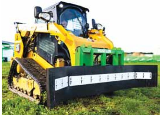
Blade and headstock's slim profile keeps the weight near the tractor for better maneuverability in tight feed pads and dairy sheds.
