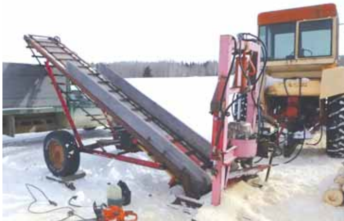
Torwalt built a log splitter and conveyor that operates on tractor hydraulics.
