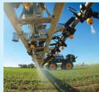
Greeneye Technology focused on row-crop agriculture in the U.S. to develop a software/hardware system that could be retrofitted on any large field sprayer. The first step was to use AI to instantly identify weeds by species.
