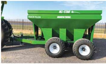
"Most of our customers use sand or gravel to minimize bridging inside the box and get the best flow out the bottom gate," says co-owner John Froese.
