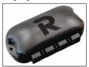
RecovR units are wireless and can be attached anywhere on equipment within minutes by magnets, self-tapping screws or with bolts.
