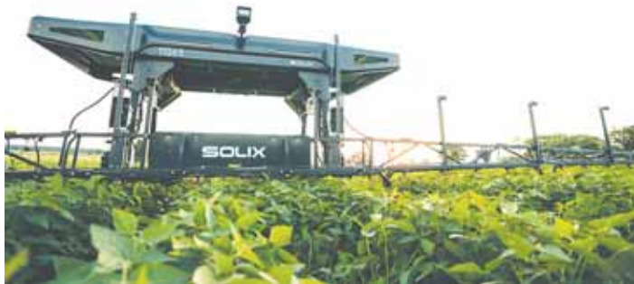
The 1,200-lb. Solix robot looks a bit like a high table on wheels with a 40-ft. boom. The chassis is 7 ft. by 7 ft. at the base.
