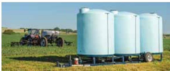
Once on site, the trailer is lowered hydraulically for filling.
