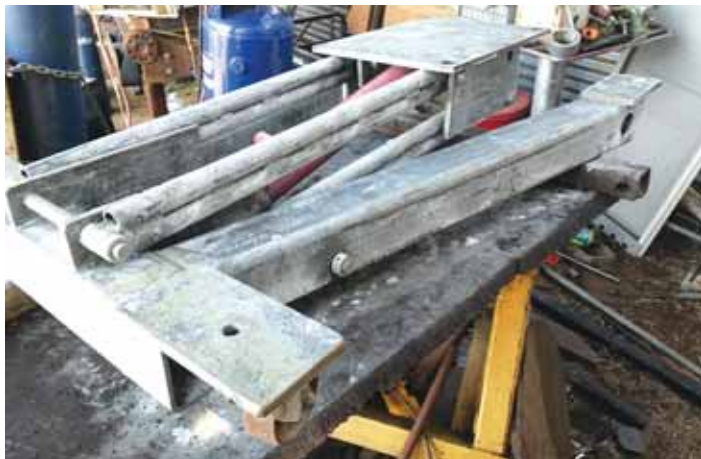
Surber built a heavy-duty transmission jack lift out of metal pieces from his junk pile and spare parts in his shop.
