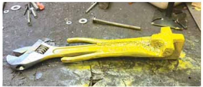
Shortridge modified an adjustable wrench to use for opening barrel bungs.
