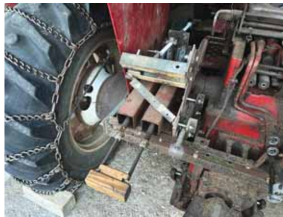
When the hydraulics fail, the rocker arm drops and the system goes to work. The springs release, unlocking the lever on the brake assembly and activating the brake drum to stop the tractor.
