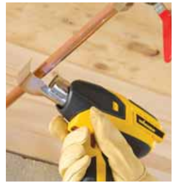
Heat gun comes with two nozzles. A flare nozzle works well for wide heat distribution, and the curved deflector wraps around a pipe.
