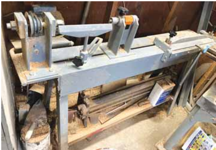
Unhappy with his wood lathe, Sieting built his own using angle iron and H-beam steel.
