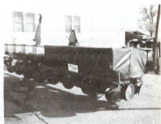
Cover is made out of vinyl coated nylon. A single cover can be used to cover as many as 6 rows at once.
