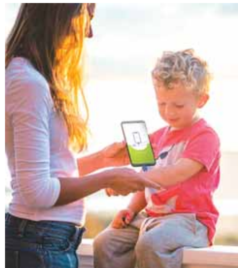
When the app signals use, the user holds it against the bite, and the affected area is briefly heated to between 117 and 126 degrees F.
