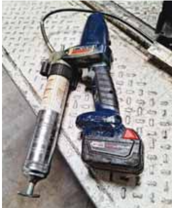
Lincoln grease gun fitted to use Milwaukee 18-volt batteries.
