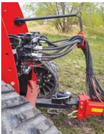
Lend-A-Hand mounts to the tractor and keeps hoses and lines up and out of the way and articulates when the tractor turns.
