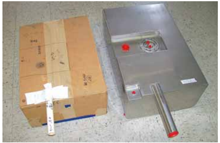
1964 Ford pickup stainless steel fuel tank with fuel injection built from a cardboard mock-up.
