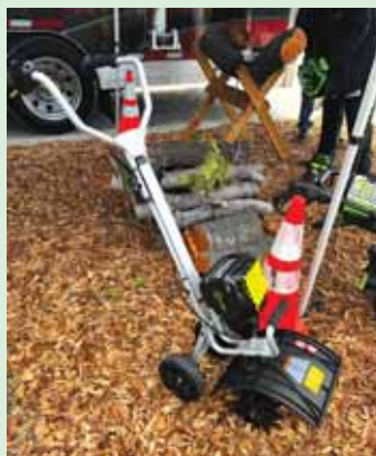
Battery powered tiller matches a 25cc gas equivalent.
