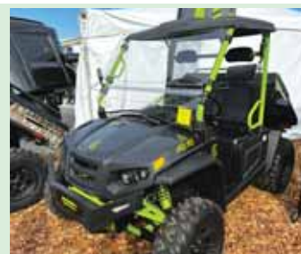
82V utility vehicle has a 1,500 lb. towing capacity and a range of up to 75 miles.
