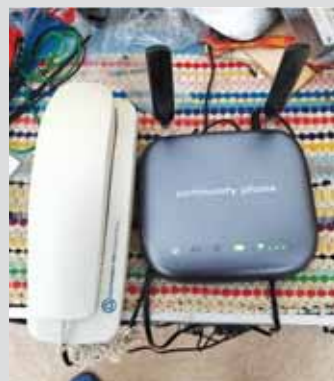
Setliff is happy with his Community Phone landline phone base that searches and locks on to cellphone signals using its external antennas.
