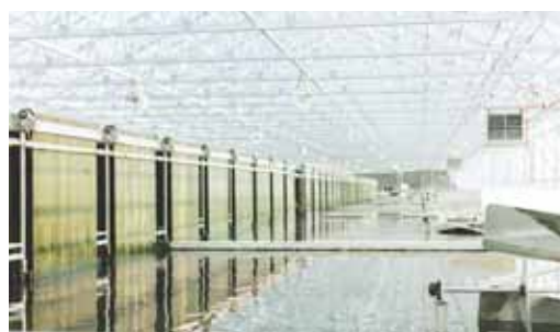
Gross-Wen Technologies originally developed their equipment to grow algae in wastewater, which they buy back, harvest, pelletize, and use to produce slow-releasing fertilizer.
