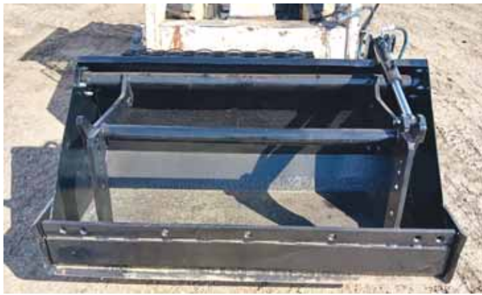
Main frame of the grapple is 3/4-in. thick steel plate salvaged from old logging equipment a friend gave McLaen. He lengthened the arms to reach the cutting edge, which was mounted to parts of an old plow.
