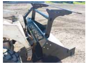
After using the bucket a few times, McLaen added a safety feature. He installed an expanded metal step to the top of the bucket.
