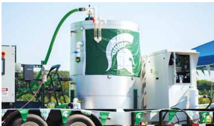
Researchers built a mobile renewable EV charging station with an anaerobic digester and external combustion engine. They also built an electric tractor to run off the power.
