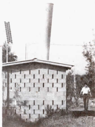
Acetylene gas explosions are projected toward hail-producing clouds by a 15 ft. cone. Solar cells at left charge the batteries.
