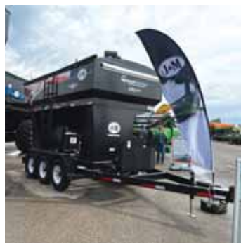
J&M EC Series SpeedTenders feature the Echo Dispense System to ensure each seed box is filled to the same level.
