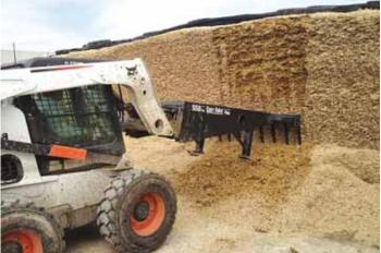
Heavy-duty tines on the end of the steel arm work like fingers across the face of the silage. The arm extends the tines out from the lift arm mechanism of the skid steer, telehandler, or payloader for greater reach.
